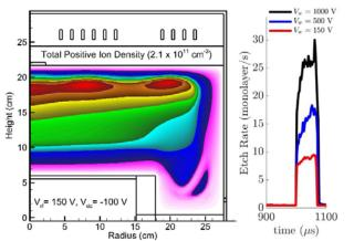
**Figure 1**. (left) Geometry of the  $Ar/Cl_2$  ICP with pulsed bias showing total positive ion density. (right) Etch rate (ML/s) for biases of 150 - 1000 V.
